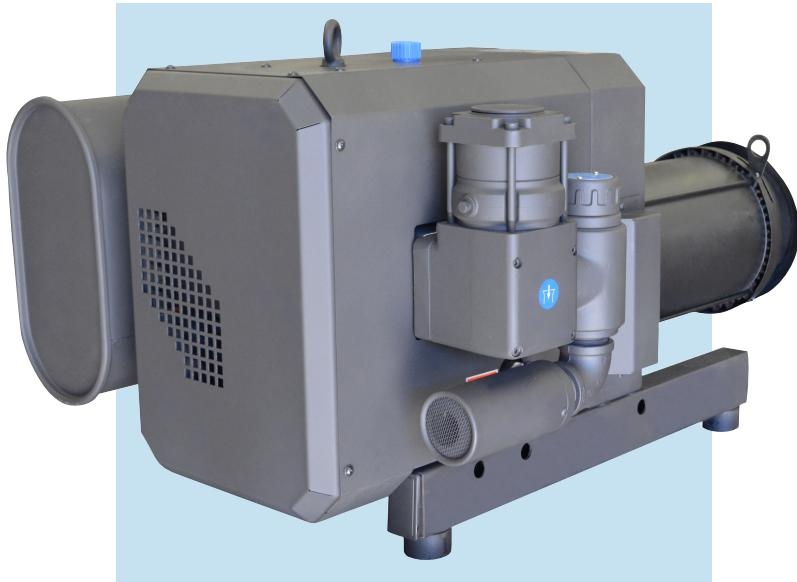
The Airtech VCX positive displacement rotary claw design is air cooled, dry-running and non-contacting. These features, along with quality construction results in a vacuum pump that is extremely high in reliability and a long service life. The non-contact design eliminates internal wear and maintenance. No water levels to check due to air-cooled operation and no sealing or lubricating oil is needed in the pumping chamber.
