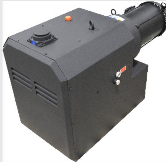
The Airtech VCX positive displacement rotary claw design is air cooled, dry-running and noncontacting. These features, along with quality construction results in a vacuum pump that is extremely high in reliability and a long service life. The non-contact design eliminates internal wear and maintenance. No water levels to check due to air-cooled operation and no sealing or lubricating oil is needed in the pumping chamber.
