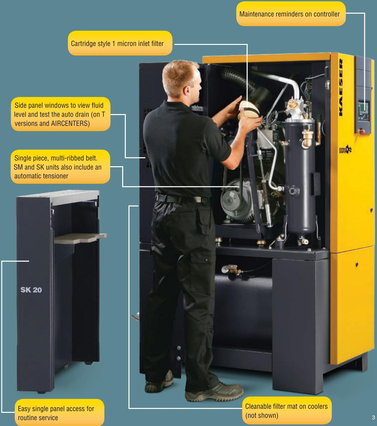
Cartridge style 1 micron inlet filter
