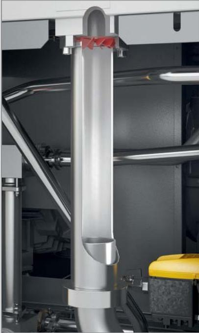
A moisture separator is integrated into the stainless steel discharge piping. Our unique design maximizes separation with minimal pressure loss—even in high ambient temperatures and humidity. A zero loss Eco-Drain is standard to automatically remove the captured moisture.
