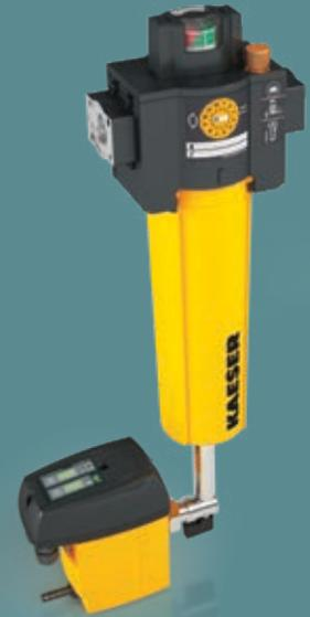
All desiccant dryers require proper filtration. Coalescing pre-filters prevent contamination of desiccant beds by hydrophobic aerosols. Particulate after-filters collect traces of desiccant dust that may exit the dryer. Maintaining these filters extends service intervals and provides excellent air quality. All Kaeser desiccant dryers offer optional filter packages with or without block and bypass valves.
