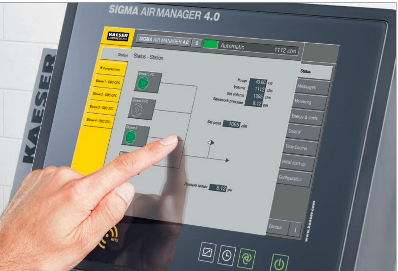
Kaeser's Sigma Air Manager 4.0 (SAM) can control up to 16 blowers and only turns them on when needed to meet air demand. This improves system stability, reduces energy use, and equalizes blower run time.
