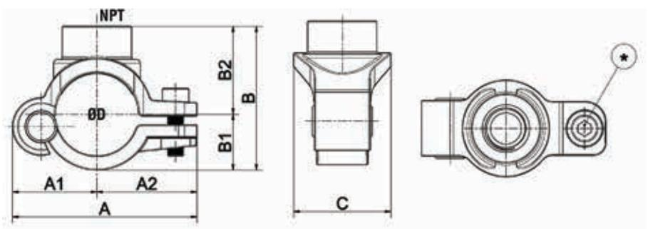
Note: Requires hole saw bit to drill pipe. 1/2" = 14 mm hole saw drill bit (ANK0043). 3/4" = 19 mm hole saw drill bit (ANK0143). 1" = 24 mm hole saw bit, includes Arbor and Pilot, (ANK0342). ANK0243 Drill arbor and pilot bit also required
