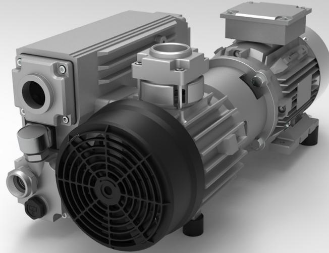
Airtech's L-Series rotary vane oil-flooded vacuum pump is a real workhorse. Reliability and durability are ensured by its simple design. Our L-Series Pump has integral exhaust filters, vibration isolators, and composite vane material which promotes longevity. The Airtech pump has an operating capacity range of 7-460 CFM while obtaining an end vacuum of 0.5 Torr.
