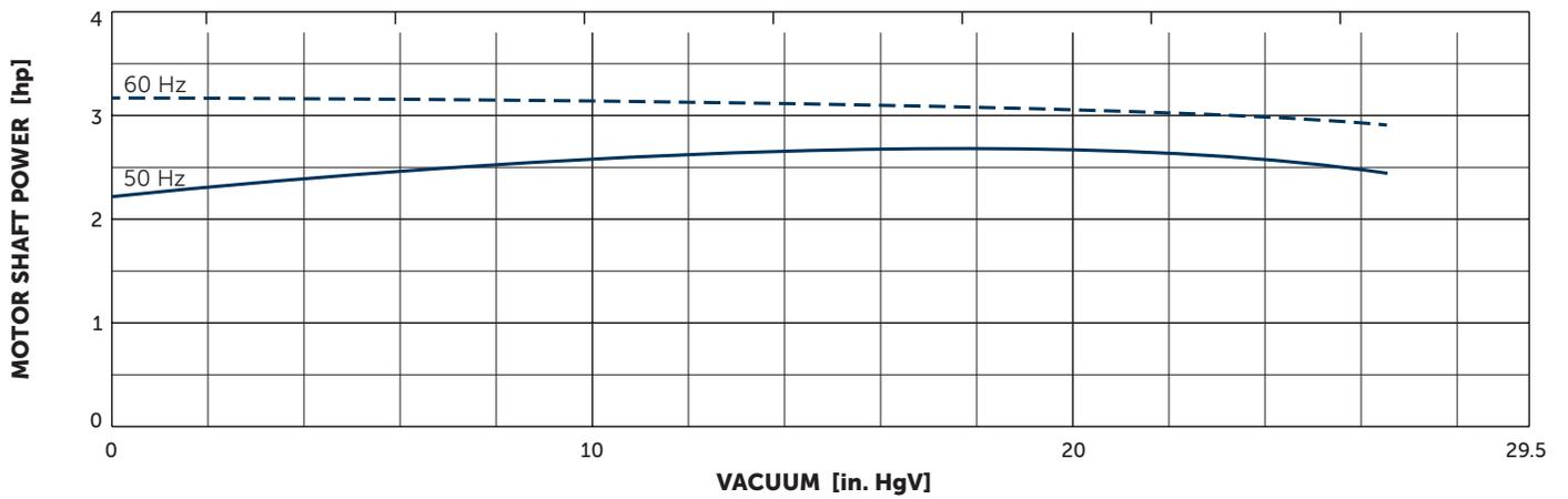
Reference data (atmosphere): 0 in. HgV, 68°F; Tolerance: ±5%
