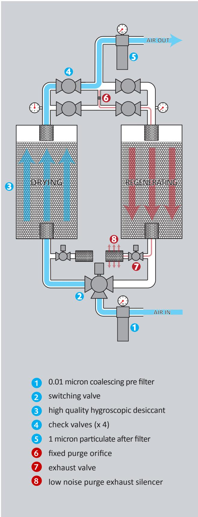
The advanced nano D-Series<sup>4</sup> high pressure compressed air dryers use the pressure swing adsorption principle to efficiently dry compressed air.
