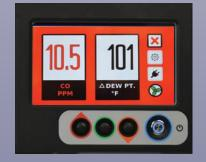
Record Keeping - In all safety air monitoring applications, keeping records is critical for OSHA compliance. With AirGuard this occurs automatically every time it is powered up. AirGuard collects a comprehensive data log recording both "Carbon Monoxide" and "Differential Dew Point" values, calibration events and diagnostic data on performance. This data is downloadable to a PC from a removable USB drive.
