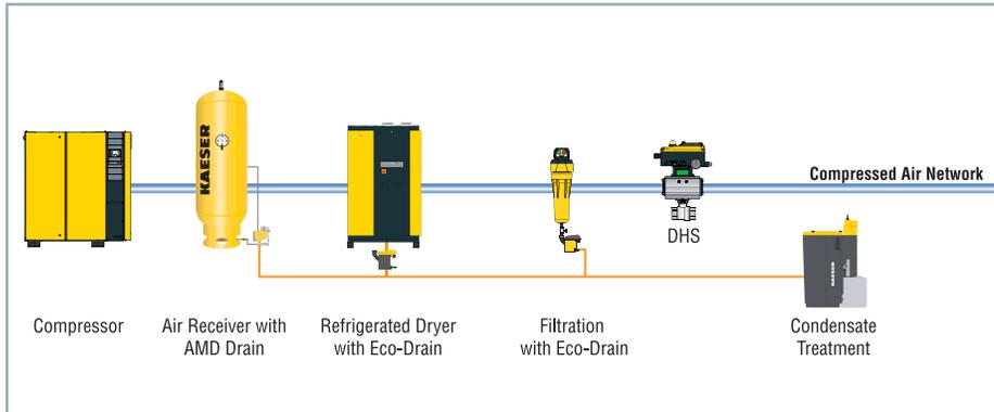
In its default configuration, the air main charging valve (DHS) is pre-set to close. If demand exceeds supply, pressure falls below the set point, or in case of power outage. It minimizes the exposure of high velocity air at start up and maintains air supply side pressure. For systems which are shut down frequently, this option further minimizes periods of high velocity air.
