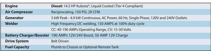
Air N Arc® 150 Diesel Unit Dimensions: Foot Print (In.): 47.0L x 21.0W x 37.6H With Fittings (In.): 48.2L x 21.0W x 37.6H Dry Weight (Lbs.): 535
