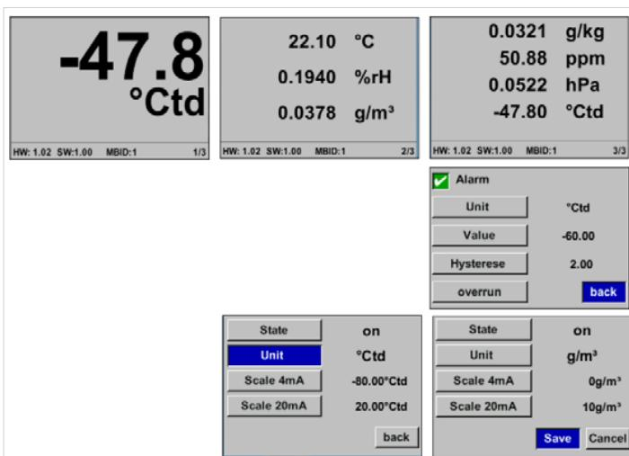
The integrated display shows the dew point in big figures as well as further humidity parameters on two more display pages. The arrow key can be used to scroll between the display pages.
